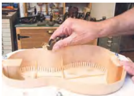
STEP 28. Trimming the sides with a thumb plane
